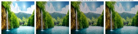
Figure 7: The model trained on 256x256 images compared to Gaussian convolutional method on Salt and Pepper noise.
